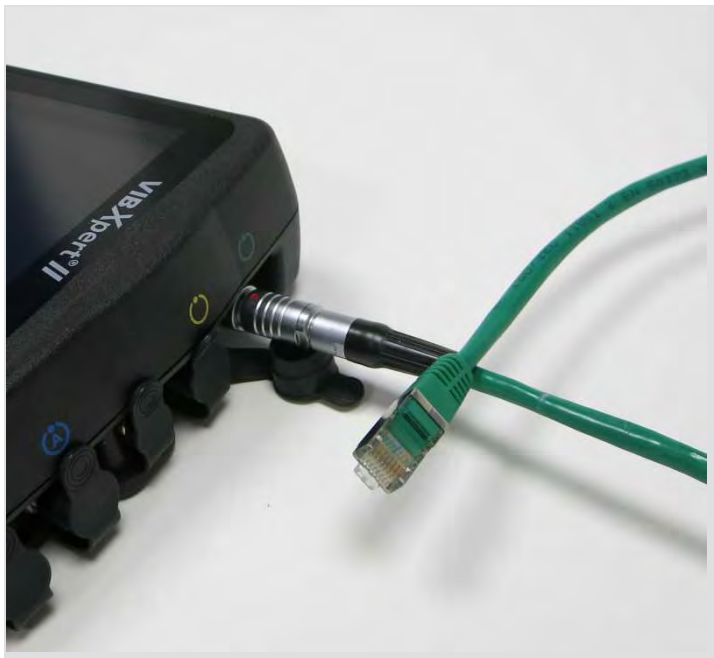
Ethernet cable connected to VIBXPERT II
