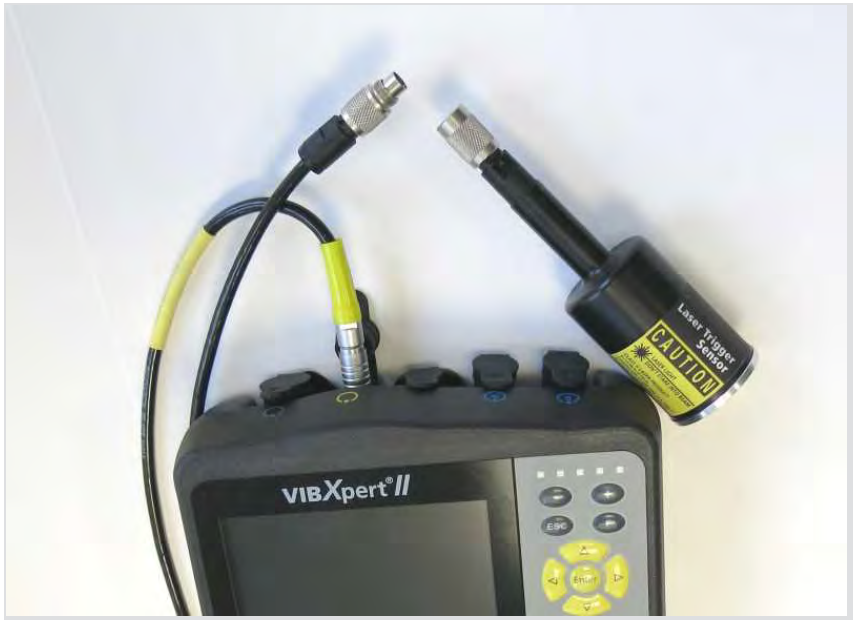
Sensor cable for laser trigger / RPM sensor VIB 6.631 connected to VIBXPERT II
