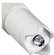
Figure 4 ORP electrode with notched body
