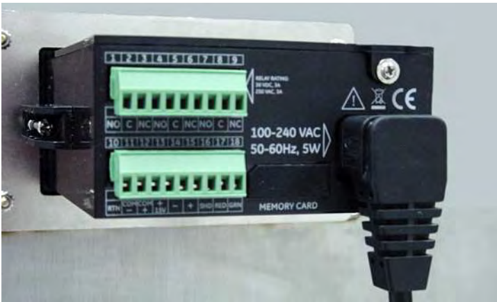
Figure 32: The AC Power Cable Installed
