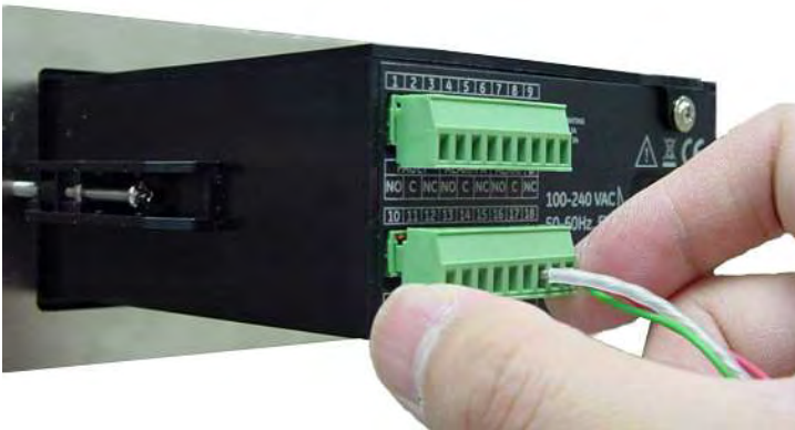
Figure 25: Reinserting the Connector into the Terminal Block
