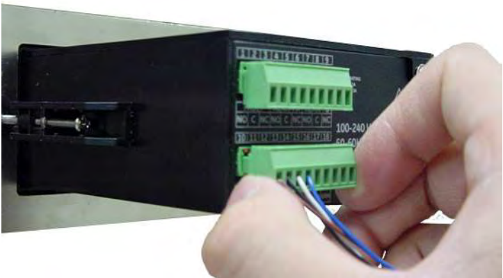
Figure 29: Reinserting the Connector into the Terminal Block
